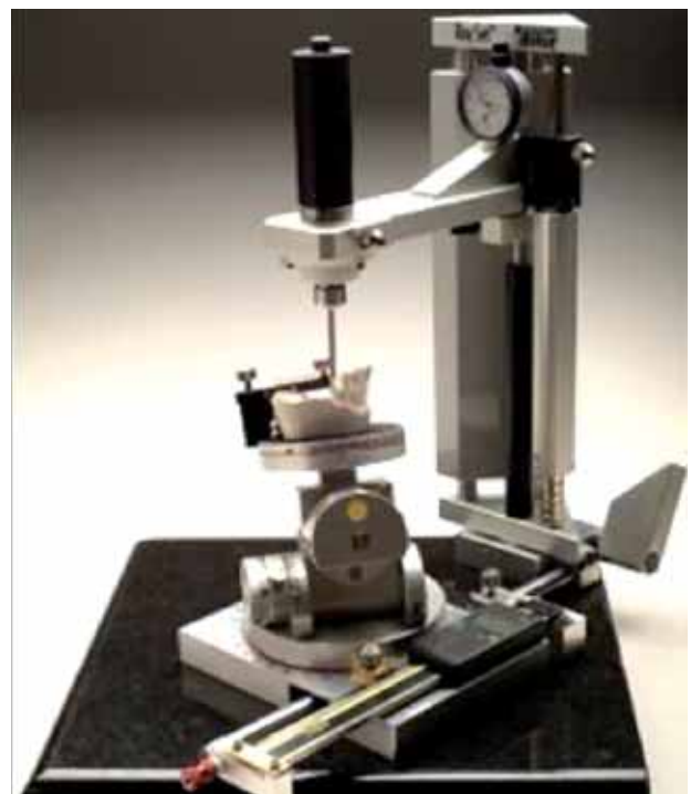
Fig. 5 The three-dimensional parallelometer for the transfer of implant position from the virtual project to the master model.
