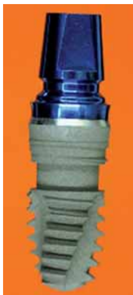
Fig. 1 Implant design. All the implants had the same basic form and topography (grit-blasted/acid-etched), but possessed four different surface coatings performed in the indentations that were placed at 2.3mm from the top with a depth of 0.18mm and a height of 1.5mm.
