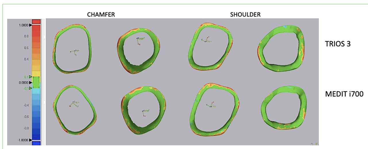
FIG. 5 Color-coded map of the marginal trueness on molars and incisors with chamfer and shoulder preparations
