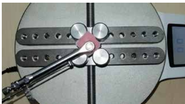
FIG. 2 Reverse torque analysis of the titanium implants (MARK-10 MTT01-12, Copiague, New York, USA).
