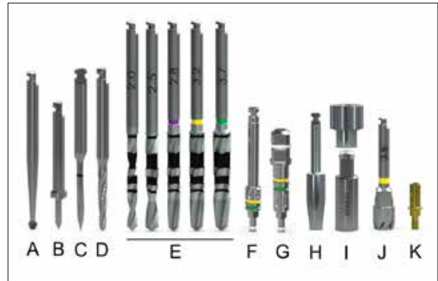
FIG. 4 Surgical instrumentation for site preparation and placement of the pterygoid implant which includes: #6 round bur (A), alignment drill (B), 1.5 mm starter drill (C), Lindemann drill (D), osteotomy drills in 2.0, 2.5, 2.8, 3.2 and 3.7 mm diameter (E), handpiece driver (F), ratchet driver (G), drill extender (H), 4 mm square drive extender and hand wrench (I), deep bone profiler (J) and bone profiler guide pin (K).
