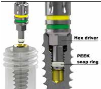
FIG. 10 The handpiece and ratchet drivers have a hex that locks into the internal hex in the PTG implant with a PEEK snap ring that frictionally connects the driver and implant preventing the implant from falling off the driver while carrying it to the prepared site intraorally.
