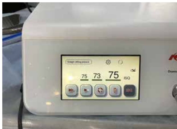
FIG. 4 ISQ values shown on the physio dispenser.
