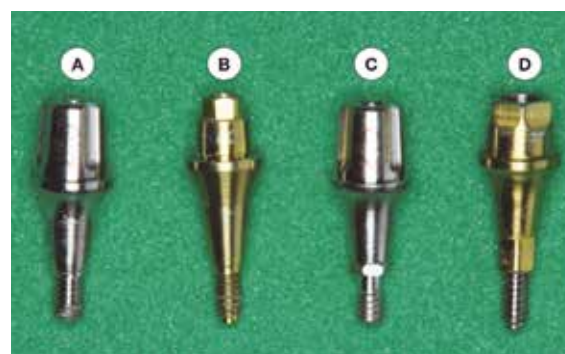
FIG. 1 A: One-piece abutment (Group 1). B: One-piece abutment (Group 2). C: Two-piece abutment (Group 3). D: Two-piece abutment (Group 4).
