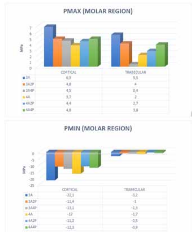
FIG. 6 Pmax and Pmin stresses occurring on the bone surrounding the implant against the forces applied against forces from molar region.
