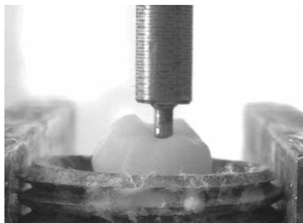
FIG. 4 Static load at fracture: axial load direction and application.
