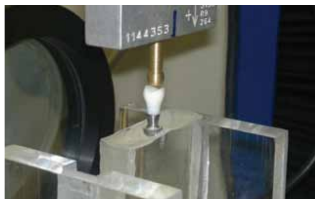
FIG. 3 Photoelastic model placed in the universal testing machine to receive the axial load at the center of the occlusal aspect.
