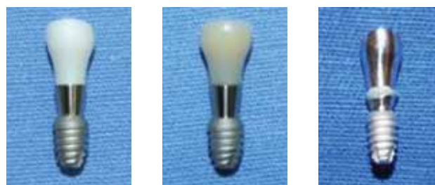
FIG. 2 Specimens composed of short locking tapered implants, universal titanium abutment and Y-TZP (left), acrylic resin (middle) and CoCr (right).
