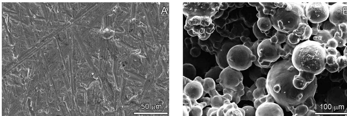
**Fig. 1** High resolution scanning electron micrographs of the dense Ti (D-Ti) and the porous-coated Ti (PC-Ti). The D-Ti surface (A) showed a slight roughness with some cutting lines. The PC-Ti structure (B) exhibited a unique topography characterized by a network of spherical particles.
