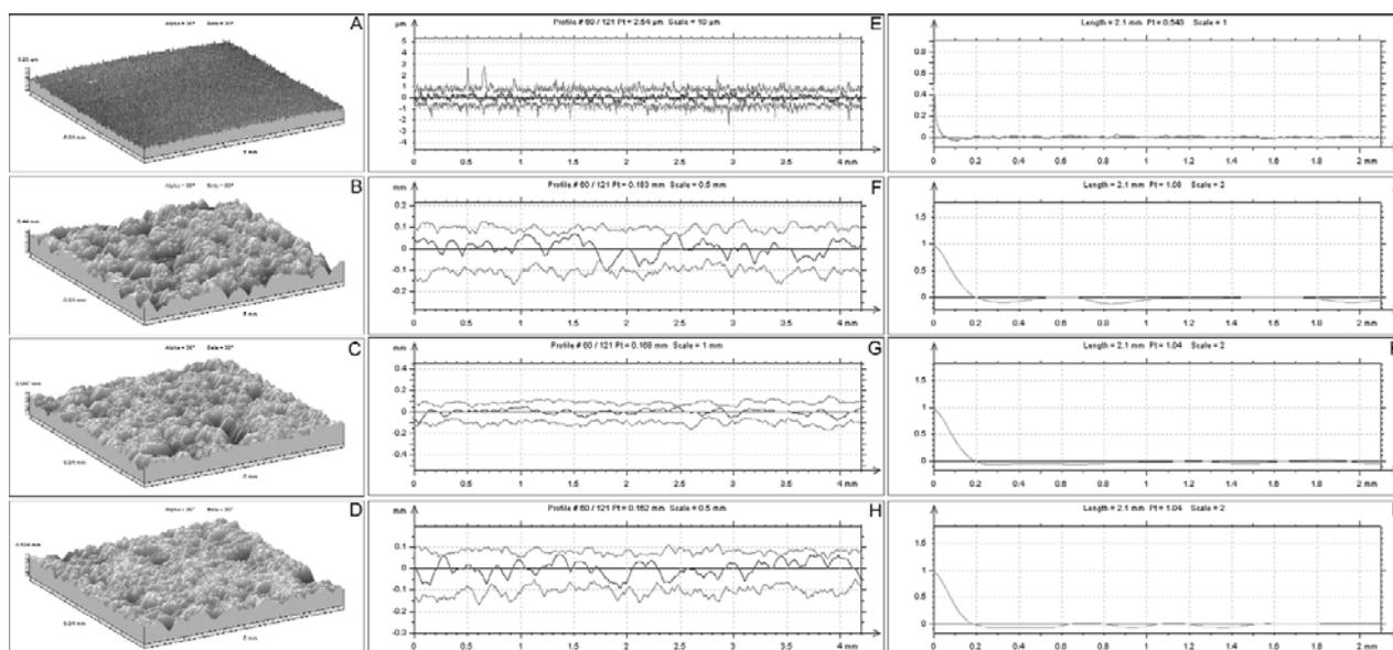
**Fig. 2** Computer generated surface images, original roughness profiles and autocorrelation function profiles for dense Ti (D-Ti) and porous-coated Ti (PC-Ti) surfaces. D-Ti (A, E and I), scale profiles ( $\mu\text{m}$ ); Porous-coated 0.5 mm (PC-0.5 - B, F and J), scale profiles (mm); Porous-coated 1.0 mm (PC-1.0 - C, G and K), scale profiles (mm); Porous-coated 1.5 mm (PC-1.5 - D, H and L), scale profiles (mm).
