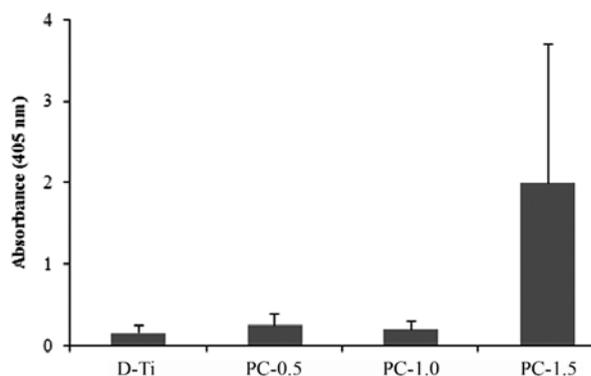
Fig. 5 Calcium content extracted from mineralized extracellular matrix of osteoblastic cultures grown on dense Ti (D-Ti) and porous-coated Ti (PC-Ti) for 17 days. The amount of calcium was significantly greater ( $p < 0.05$ ) on porous-coated 1.5 mm (PC-1.5) surface compared to all other Ti surfaces. Data are reported as mean ± standard deviation ( $n = 4$ ).
