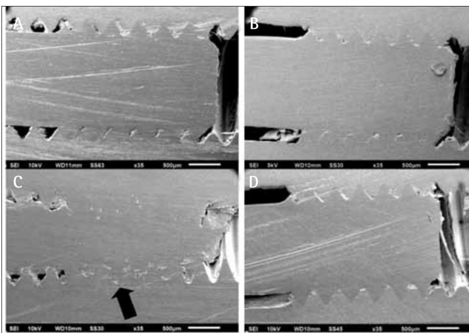
FIG. 2 SEM images of the implant/abutment/screw assemblies at a 35X magnification. A: Conventional EH before loading; B: Internal torque EH before loading; C: Conventional EH after loading; D: Internal torque EH after loading.
