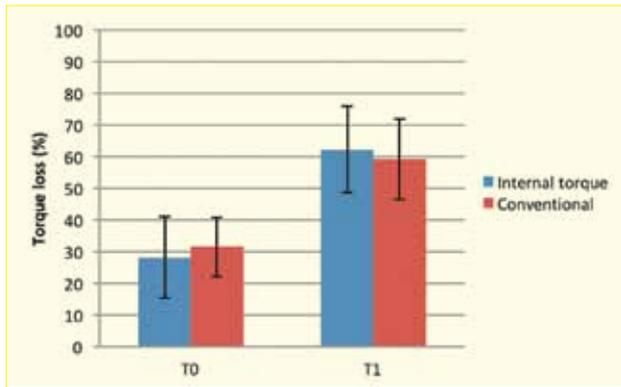
FIG. 1 Percentage of torque loss of conventional and internal torque implants, before and after cyclic loading.
