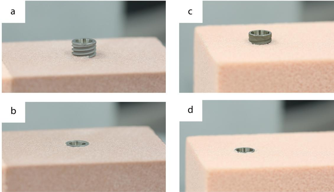
FIG. 4 Implant placed with 32 Ncm in bone type I (a). With final torque (b). Implant placed with 32 Ncm in bone type IV(c). With final torque (d).
