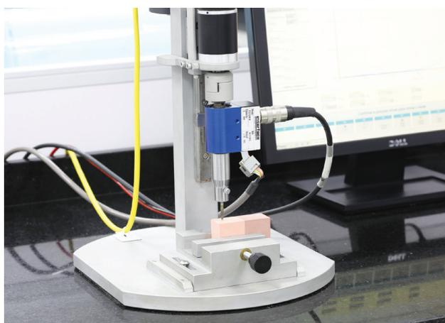
**FIG. 3** Implants placed by the Multi-Functional Twisting Machine.
