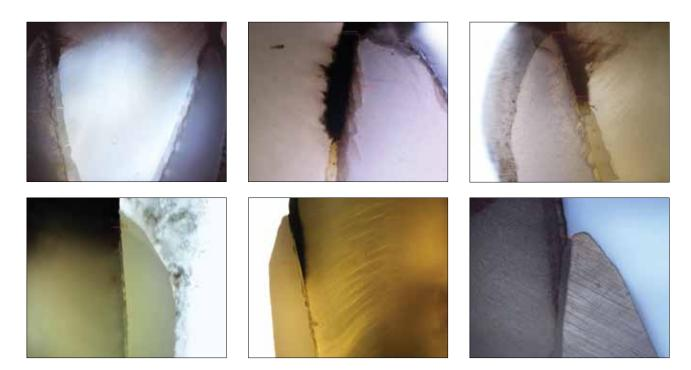
FIG. 16 Microscopic images showing nanoleakage of a lithium disilicate (16a-16c) and of a zirconia crown (16d-16f).
