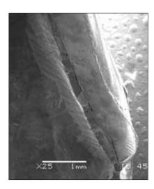
FIG. 14 SEM images (14a: sample crown before cutting at 25x; 14b-14c: two margins of lithium disilicate crowns showing fractures at 65x and 350x; 14d-14e: two intact margins of zirconia crowns at 130x).
