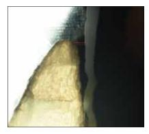
FIG. 15 Microscopic images showing fractured margins of lithium disilicate crowns (4x, 10x). differences among the four cements inside each group of crowns but there were significant differences between zirconia and lithium disilicate crowns (Table 4). Marginal gap
